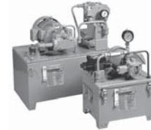
**NCP Series** is a compact, low-cost standard unit that includes a variable vane pump (VDS, VDR, VDC Series) or a variable piston pump (PVS/PZS Series). The power unit is low-noise, low-heat, energy-efficient, and highly reliable. The NCP Series has been expanded to include a choice of models that are optimized for a very wide range of needs. Available tank capacities range from 30 l to 650 l.
